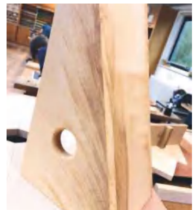
▲ Pic.36 The drawer handle is a hole. There is also a smaller hole in the back panel to allow the drawer to open freely and not get stuck due to vacuum. I thought the figuring of the rippled sycamore worked really well here. I then used a pillar drill and a hand-held router to round off the edges
